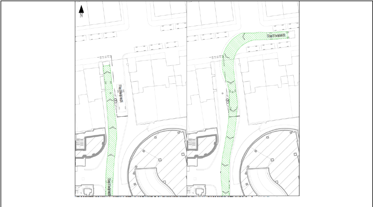
Figure 10: Proposed Almeida Street access showing swept path vehicle tracking for a 10m rigid van.
